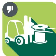
It is essential to **avoid** lifting and transporting a loaded plastic reel on the outside of the flange
