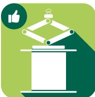
**Horizontal reels** may only be picked up and transported positive-locked via the spindle hole (central bore) with a suitable and approved load handling equipment (reel lifter, internal gripper).
