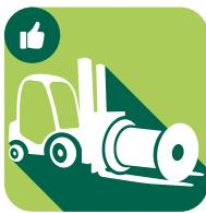
**Vertical reels** must be secured against rolling away unintentionally and may only be transported using suitable lifting and transport systems. Lifting and transporting vertical reels is only permitted via both flanges at the same time. Avoid rolling the reel on the flange edges for longer distances.
