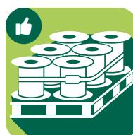
Loaded and horizontally stored reels must be palletized and strapped.
