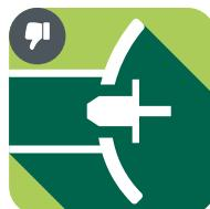
**Note:** If the diameter of the pressure flange is smaller than the diameter of the core hole, the load or the contact pressure inside the core hole will be too high, which will lead to undesired deformations even to the extent of the flange tearing off.
